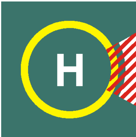
Figure 5-7. Helideck prohibited landing sector marking
